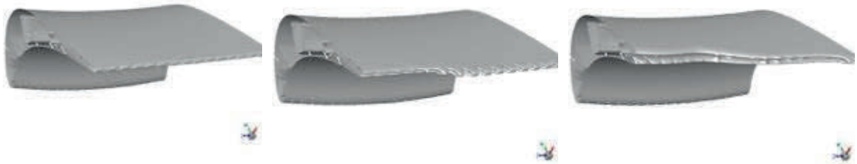
Fig.18: Stages during the simulated burn-through of the cooled turbine blade: geometry
