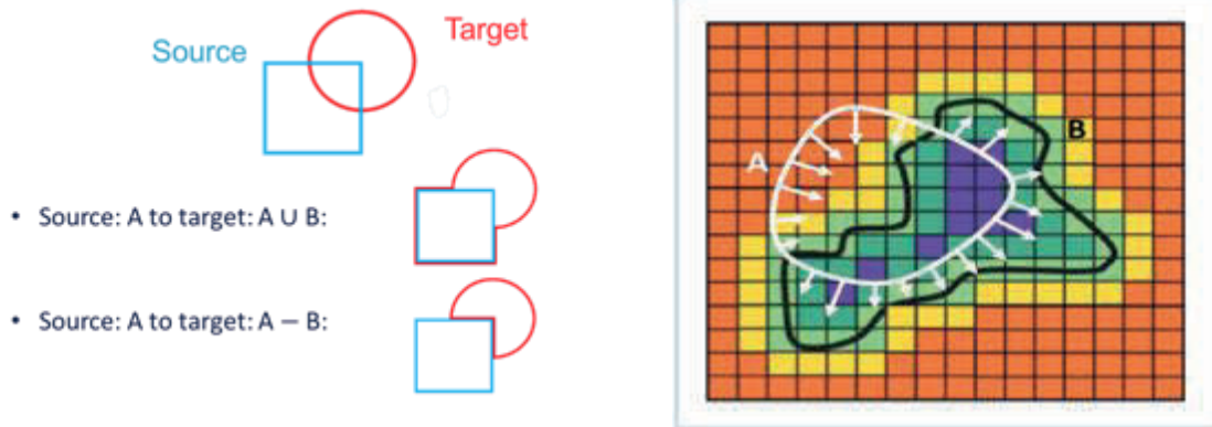
Fig.9: Digital Geometry editing the Distance Field: (left) simple Boolean operations; (right) morphing Shape “A” to Shape “B”
