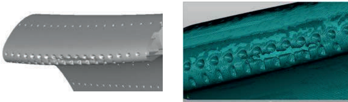
Fig.19: Geometry and associated mesh in the later stages of the burn-through simulation.
