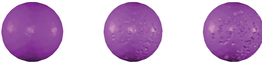
Fig.10: Stages in the erosion of a sphere subject to sand particle impingement; the image shows the zero distance of the Level Set geometry
